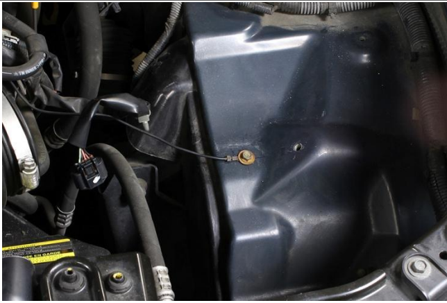
10. Unbolt the grounding wire from the frame with a 10mm socket.
