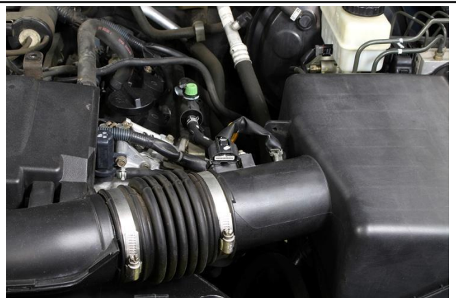
3. Unplug the connector on the MAF sensor, then unclip the harness from the air box.
