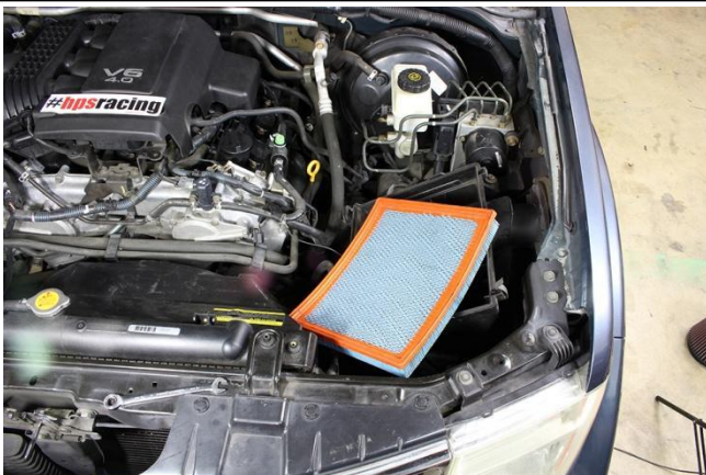
8. Remove the panel filter from the air box.
