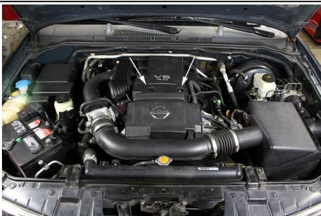
2. Unbolt the two bolts to remove the engine cover.
