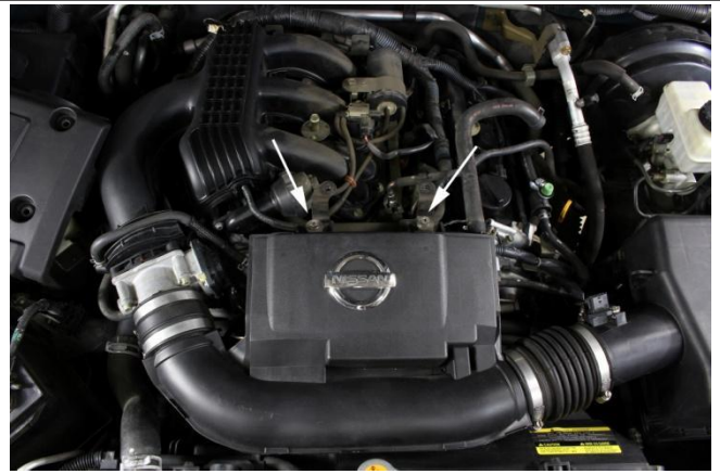
5. Remove the two bolts securing the crankcase ventilation box.
