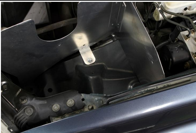
12. Use another M6 bolt and washer to secure the base of the heat shield at the original grounding point in Step 10.
