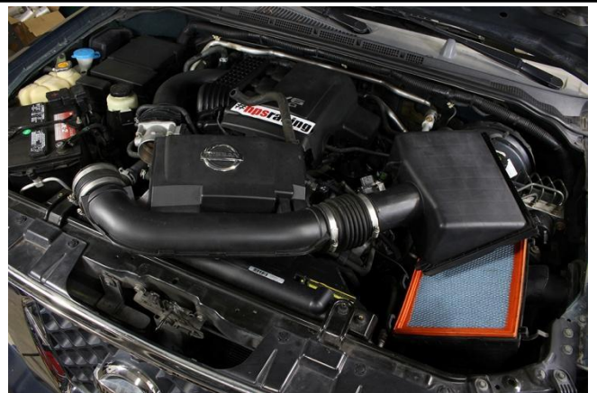
7. Unbuckle the upper air box cover, and remove the intake assembly as one piece.
