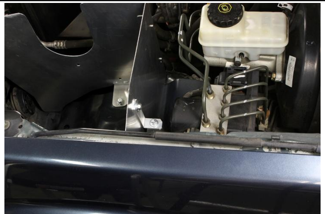
13. Install the heat shield bracket onto the stock air box mount located near the ABS unit using a M6 bolt and washer. Secure the other end using a M6 bolt, washer, and nut.
