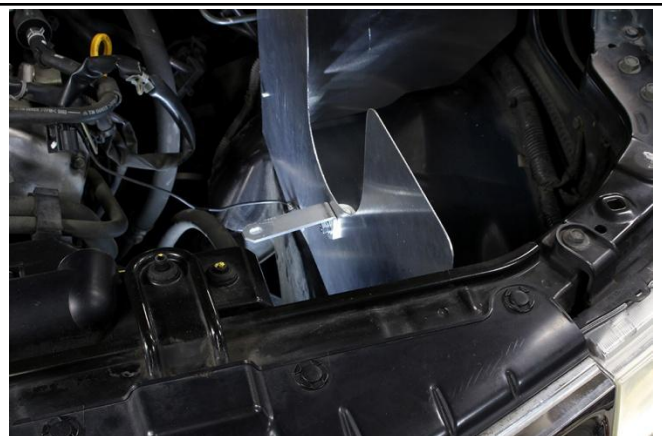
15. Install the intake mounting bracket onto the heat shield at the semi-circle opening using a M6 bolt, washer, and nut.
