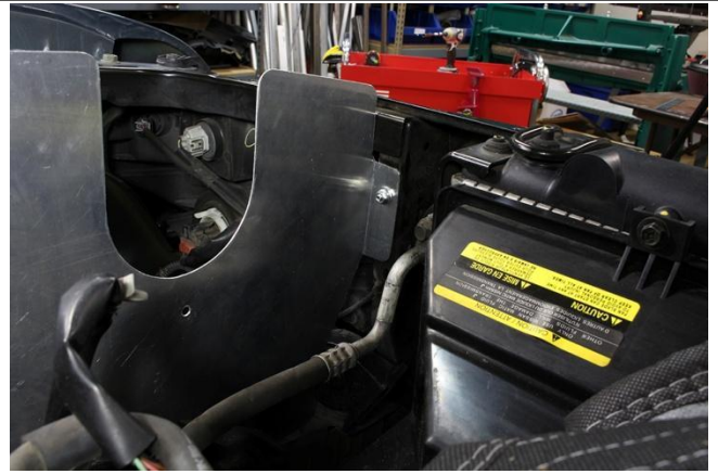
11. Begin installing the heat shield. Use the provided M6 bolt along with a nut and washer to secure the heat shield to the radiator support.
