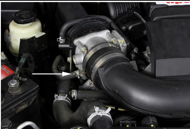
6. Use a flat head screwdriver to loosen the clamp securing the intake pipe to the throttle body.
