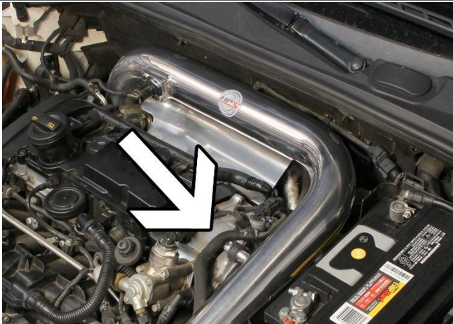
12. Align the vibration mount onto the mounting location as indicated, then press the intake pipe into the coupler on the turbo inlet. Tighten the T-bolt clamp.
