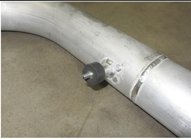
10. Install the rubber vibration mount onto the intake pipe.
