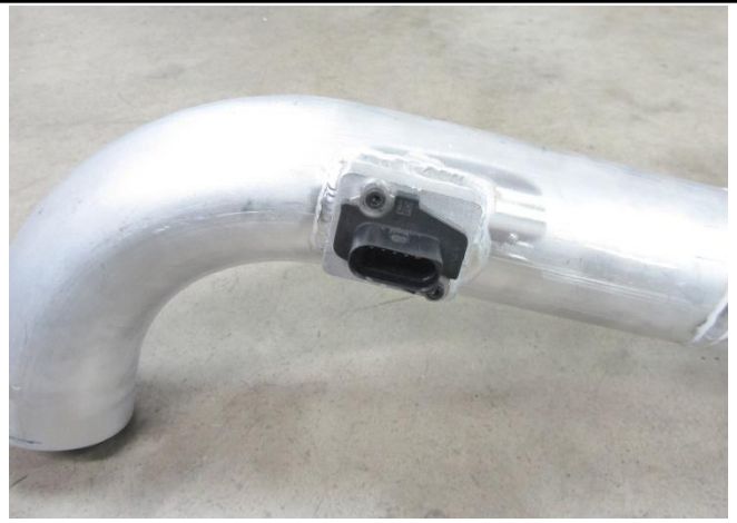
11. Transfer the MAF sensor onto the HPS intake pipe and secure it using the 4mm allen screws provided in the hardware pack.
