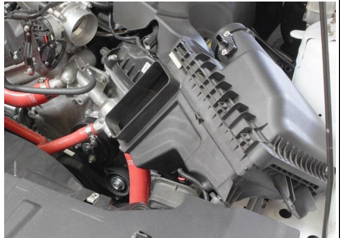
7. Remove the airbox from the engine bay.
