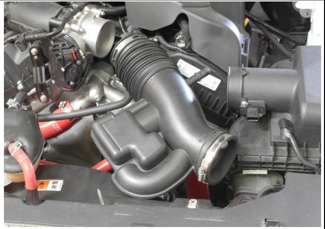
5. Remove the factory air tube from the vehicle.
