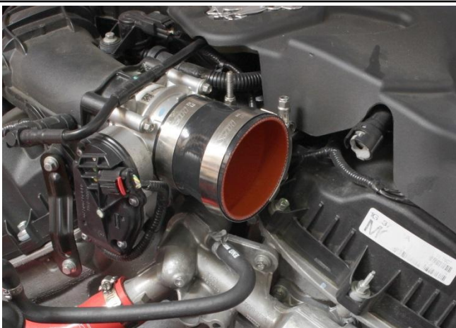
8. Install the silicone coupler onto the throttle body along with the two T-bolt clamps.
