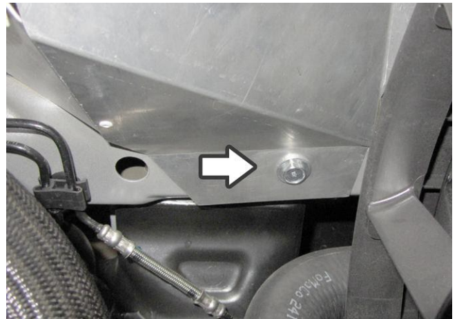
13. Secure the bottom mounting location with the M8 bolt and washer provided.
