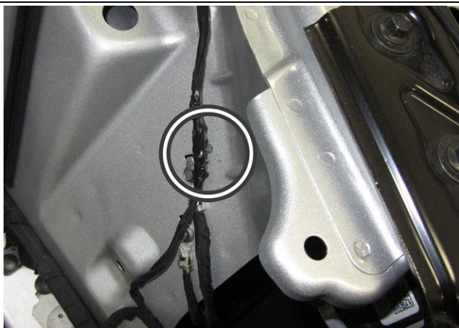
14a. Remove the tab connectors holding the MAF harness from the locations shown.
