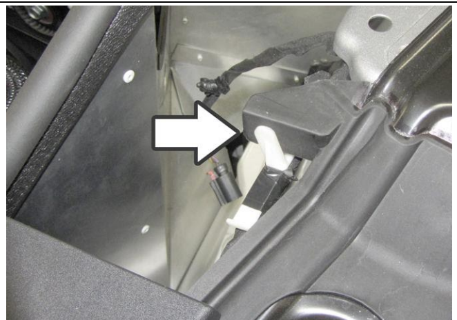
14b. Remove the tab connectors holding the MAF harness from the locations shown.
