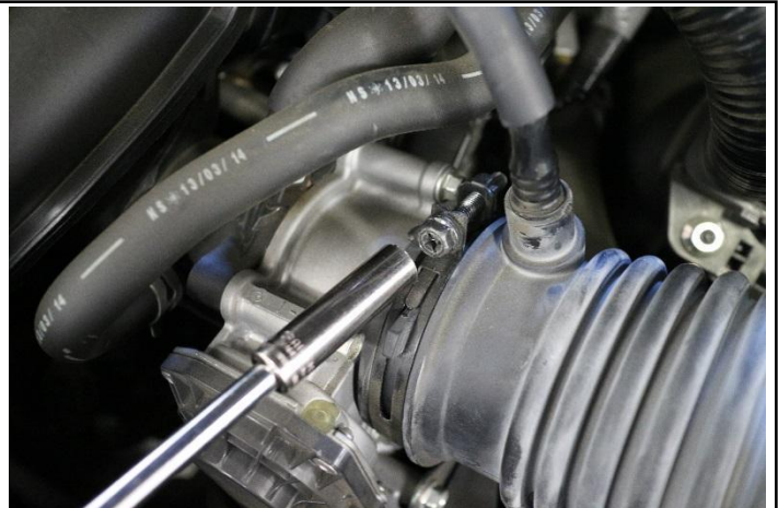
3. Loosen the hose clamp on the throttle body using a 10mm socket.
