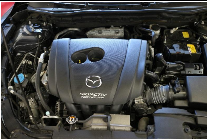
2. Remove the engine cover by pulling up on the 4 corners.
