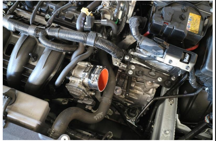
9. Install the silicone reducing coupler and T-bolt clamps onto the throttle body.
