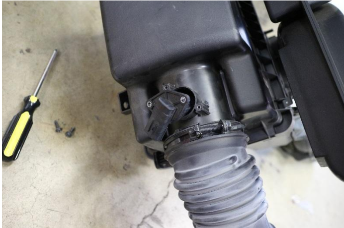
10. Use a phillips head screwdriver to remove the MAF sensor from the air box. Be careful not to damage the sensor.
