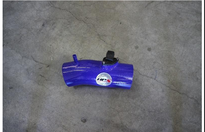
11. Transfer the MAF sensor to the HPS intake pipe, then use the supplied allen screws to secure it to the pipe.
