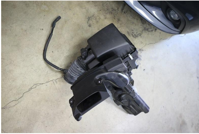
8. Disconnect the intake tube from the throttle body then lift up on the air box to remove it from the engine bay.
