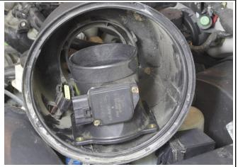
9. Disconnect the harness from the mass air flow sensor. Keep the MAF sensor in a safe place as it will be needed again later.
