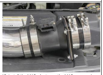
15. Install the MAF adapter on the MAF sensor using the hardware provided, then install a coupler on both ends of the sensor as shown in the picture.
