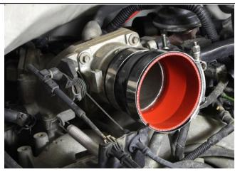
11. Press the silicone coupler onto the throttle body, along with the two T-bolt clamps. Only tighten the clamp on the throttle body for now.
