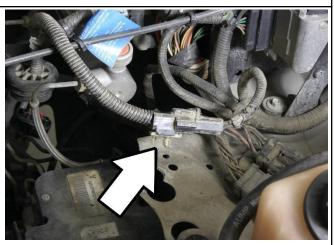
\*13. Vehicles equipped with cruise control remove the harness to install heatshield.
