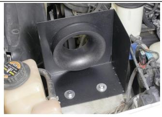
14. With the factory rubber grommets in place, sandwich the heatshield on using a bolt and washer on the top, then a washer and nut to secure it at the bottom.
