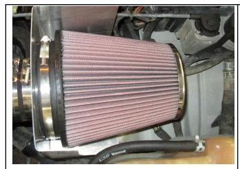
22. Insert and secure the HPS air filter onto the velocity stack.
