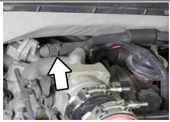
18. Disconnect and remove the breather hose located behind the throttle body.
