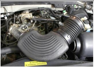
5. Loosen the clamps on the throttle body and the stock air box, then remove the factory intake elbow from the engine bay.
