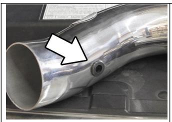
16. Install the rubber grommet included in the hardware pack onto the intake pipe and insert temperature sensor.
