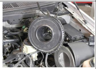
6. Unbuckle the clamp to separate the air box.
