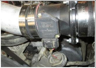
21. Reconnect the MAF sensor harness back on.
