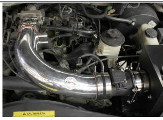
17. Insert the intake pipe into the throttle body coupler and the other side into the heatshield.
