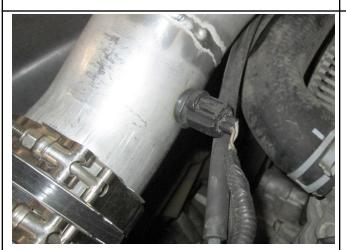
20. Install the temperature sensor onto the pipe and reconnect the electrical connector.
