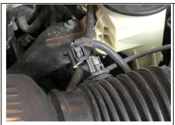
4. Disconnect the temperature sensor from the intake pipe.
