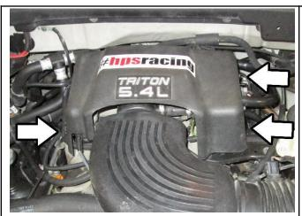
2. Remove the engine cover by unscrewing the three bolts indicated.
