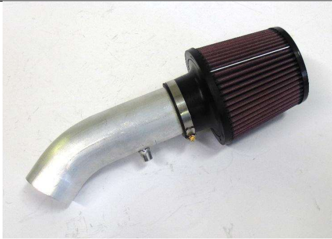
14. Install the HPS air filter onto the HPS intake pipe.
