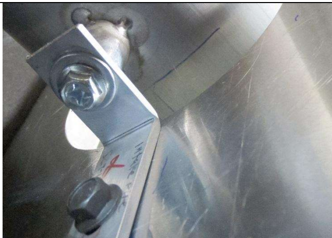
16. Bolt the intake to the intake bracket using the remaining 6mm bolt and washer.
