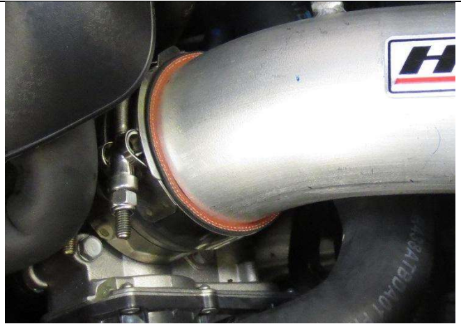
15. Install the intake pipe onto the throttle body coupler.
