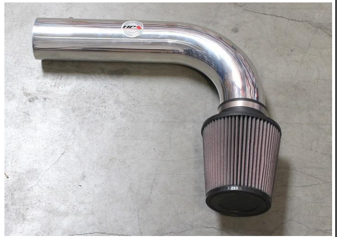
19. Install the air filter onto the intake pipe as show.
