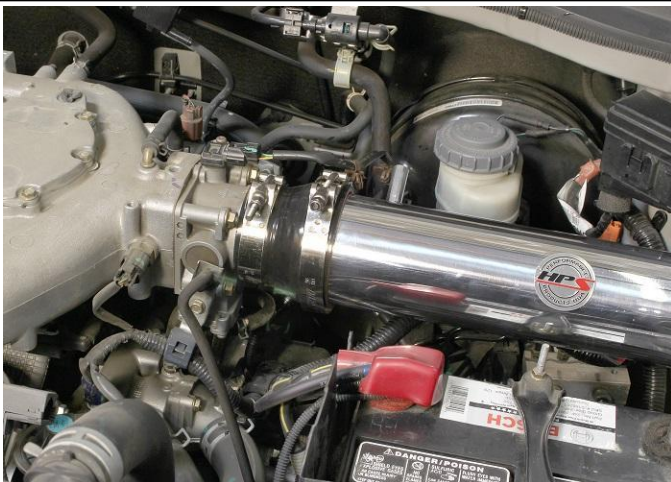
20. Place the t-bolt clamp on the large end of the silicone coupler, then press the intake pipe into the coupler.
