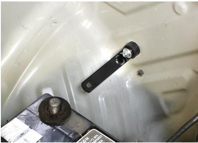
18. Loosely install the intake bracket onto the rubber mount using a 6mm nut and washer.
