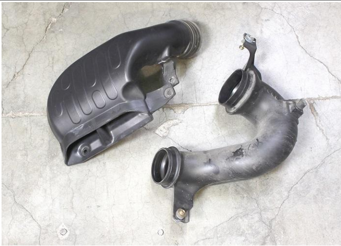
10. Remove the air scoop assembly from the engine bay.
