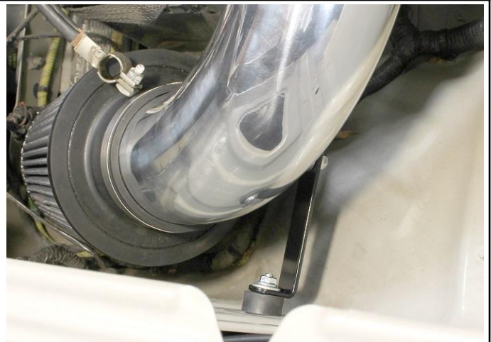
21. Attach the intake pipe onto the bracket using the m6 bolt and washer included in the hardware pack.
