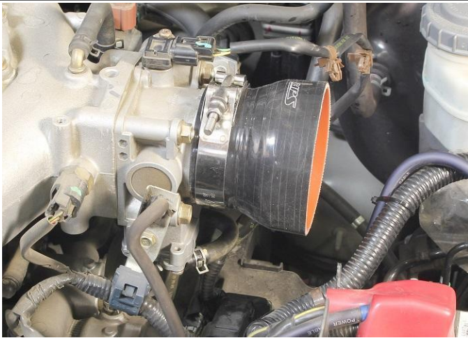
16. Install the silicone coupler onto the throttle body with the corresponding T-Bolt clamp.
