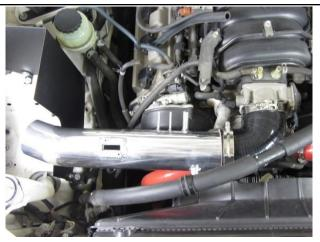
10. Install the 90° silicone elbow onto the throttle body along with a provided T-bolt clamp. Install the HPS intake pipe into the 90° elbow along with another T-bolt clamp.
