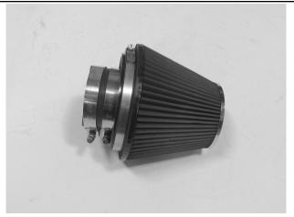
12b. Press the velocity stack into the air filter, then place the silicone copuler onto the velocity stack. Place two T-bolt clamps onto the coupler and make them snug enough that they won't fall off.
