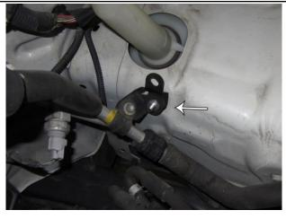
7. Replace the removed bolt from Step 6 with the rubber vibration mount included in the hardware kit.
