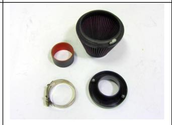
12a. Prepare the air filter for installation by assembling the air filter, velocity stack, straight coupler, and two T-bolt clamps.
