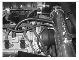
16. Replace the valve cover breather hose with the hose included in the hardware pack. Attach the vacuum lines to the HPS intake pipe as shown.
