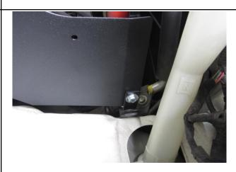
8. Install the 45° bracket onto the vibration mount using the 6mm washer and 6mm nut included in the kit.
