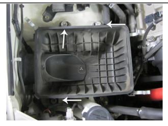
5. Loosen the 3 bolts securing the lower air box assembly with a 10mm socket, then remove the lower air box assembly from the engine bay.
