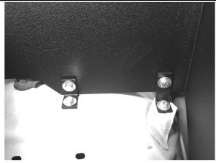
9. Install the smallest and longest brackets into the bolt holes used for the stock air box as shown using a 6mm bolt and washer for each one. Mount the heat shield onto the brackets using a 6mm bolt, a washer on each side, and 6mm nut for each one.
