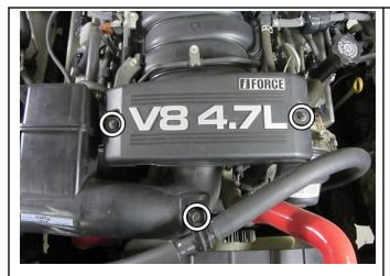
2. Remove the two nuts securing the engine cover (shown in the top two circles) using a 10mm socket, then remove the cover. Also, remove the bolt securing the power steering hose (shown in the lower circle).
