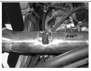
14b. Carefully insert the MAF sensor into the HPS intake pipe and secure with the provided 4mm allen screws.
