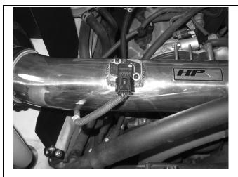
17. Connect the MAF sensor harness to the sensor.
