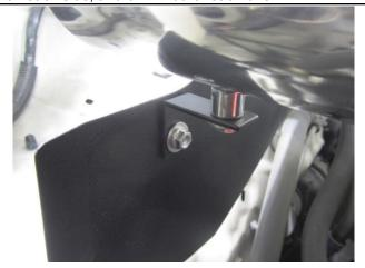
11. Secure the HPS intake pipe onto the heat shield using the medium length bracket, along with 2 6mm bolts, 3 washers, and a 6mm nut from the hardware pack.
