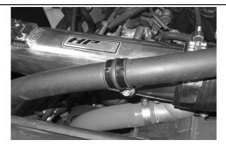
15. Remove the Adel clamp and flip it 180° (so that the flat part of the bolt hole is towards the engine and pointing down). Place the clamp back onto the hose and use a provided 6mm bolt to secure the hose to the HPS intake pipe.
