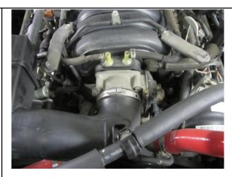
4. Use a Flat-head (blade) screwdriver to loosen the clamp securing the intake tube to the throttle body. The intake tube and upper air box can then be removed as one piece.
