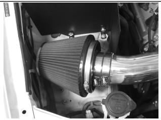
13. Press the air filter and coupler onto the HPS intake pipe, and tighten the T-bolt clamps.
