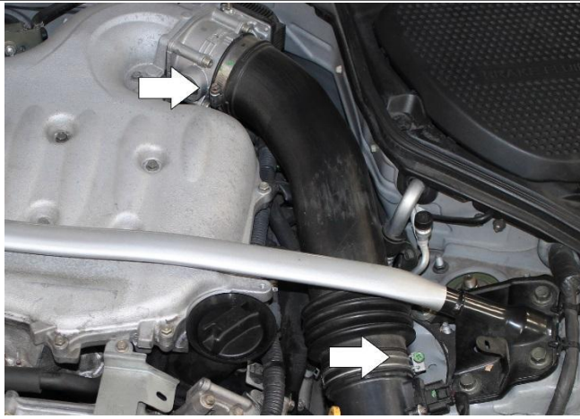
4. Loosen the clamps securing the intake pipe to the throttle body and the MAF sensor housing.
