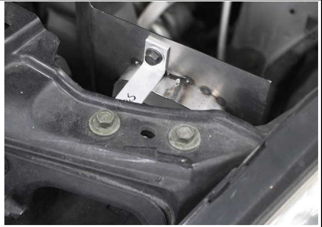
23. Slide the L bracket in between the radiator support and reinstall the bolts. Secure the heat shield to the bracket using a M6 x 12 bolt and washer.
