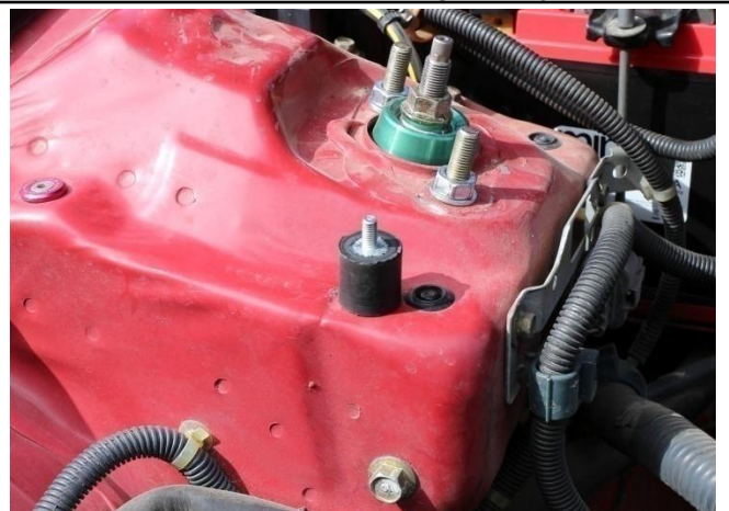
9. Install the 1" rubber mount onto the threaded hole on the shock tower.
