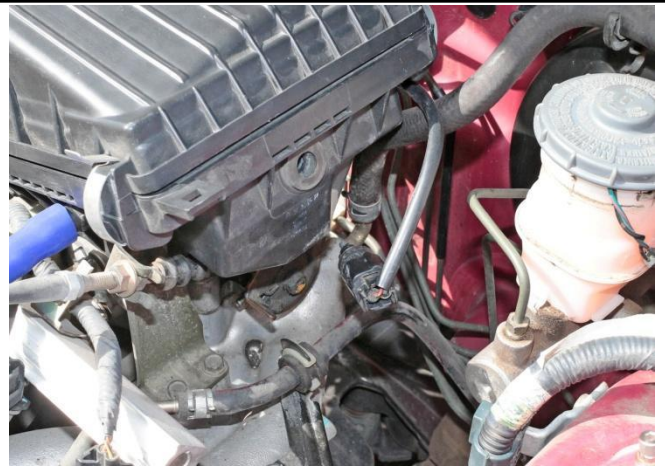
5. Remove the intake air temperature sensor from the air box.
