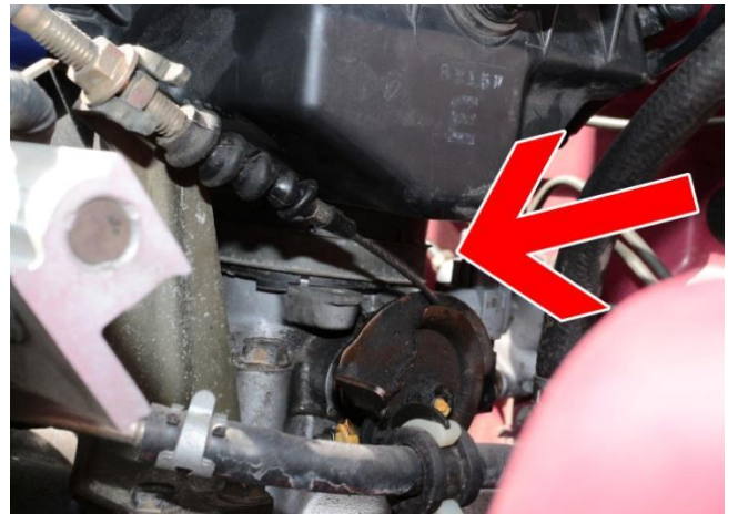
7. Loosen the clamp on the throttle body and remove the airbox from the engine bay.
