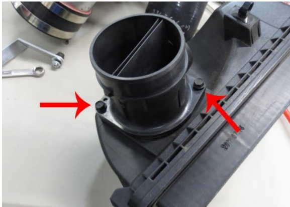
12. With the air box removed from the vehicle, Disconnect the MAF housing from the air box by removing the 2 bolts. When the MAF housing is removed from the air box, remove the rubber o-ring from the MAF housing.
