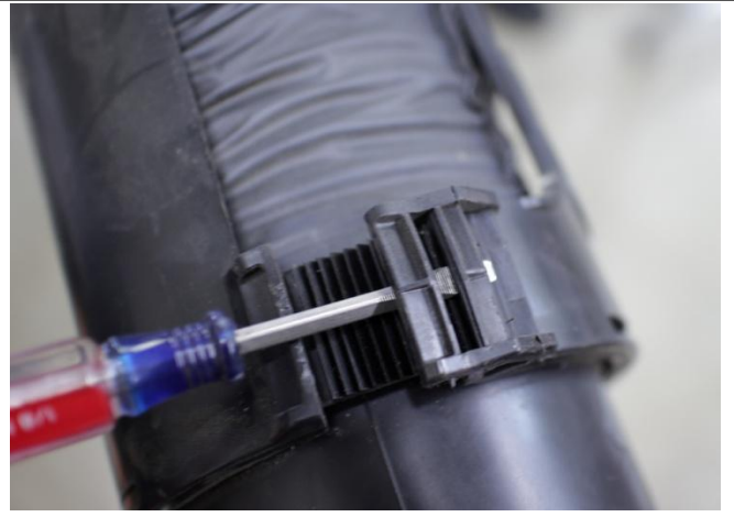
17. Optionally, you can reinstall the air duct. The factory air duct hose has a glued connection. Some parts may not be reused after disassembly.
