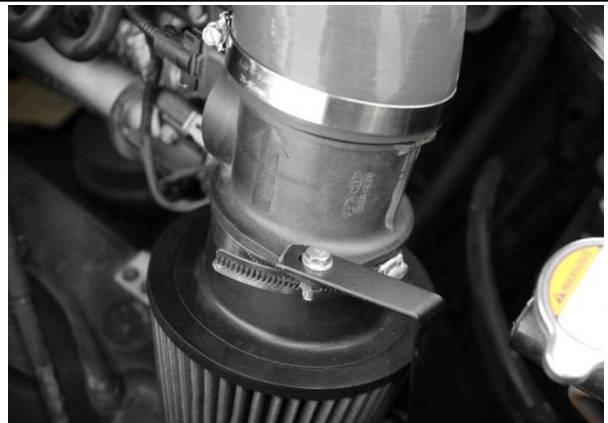
15. Clock the MAF housing until the bracket lines up with it. Install the long bolt with the included washers and nut, then tighten down. Once the bracket is secured, you can tighten the clamps on the silicone elbow. Reconnect the MAF harness.
