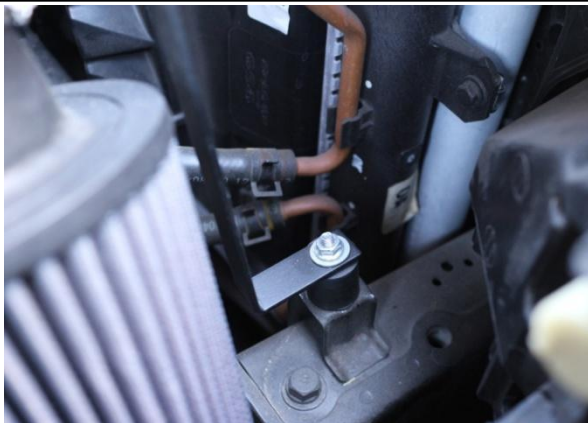
14. Install the rubber mount onto the factory air box mounting location. Place the bracket onto the rubber mount and secure it with a nut and washer included in the hardware pack.
