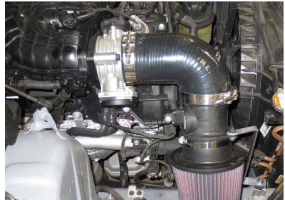
13. Install the silicone elbow onto the throttle body and loosely fit the clamps onto it. Connect the MAF housing to the silicone elbow with the sensor connector facing approximately at the 10 o'clock position. Then install the air filter onto the MAF housing.
