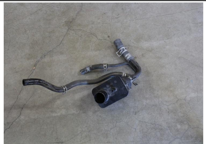
9. Remove the stock coolant hose assembly from the vehicle.
