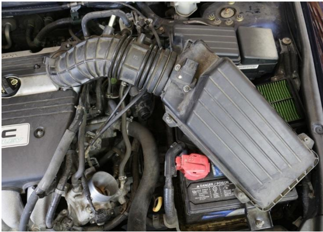
6. Pull the intake tube firmly from the throttle body and remove the top portion of the air box as well as the stock intake tube from the vehicle.
