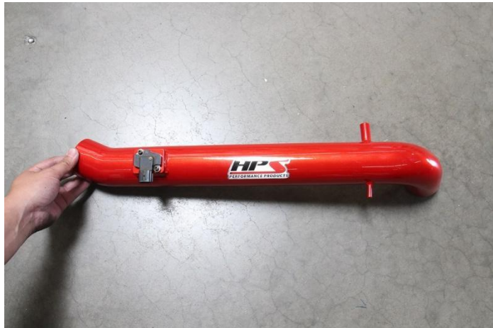
22. Install and secure the Mass Air Flow sensor onto the HPS intake pipe using the provided M4 x 8mm allen bolts.
