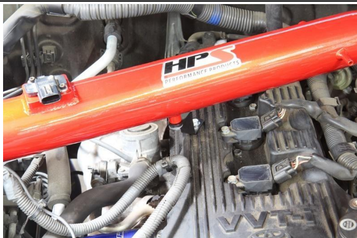
24. Align the intake bracket with the mounting bung on the intake pipe. Once, the intake pipe is aligned with the opening of the heatshield, tighten the bolts securing the bracket to the valve cover, the intake pipe to the bracket, and the T-bolt clamp securing the intake pipe to the coupler.
