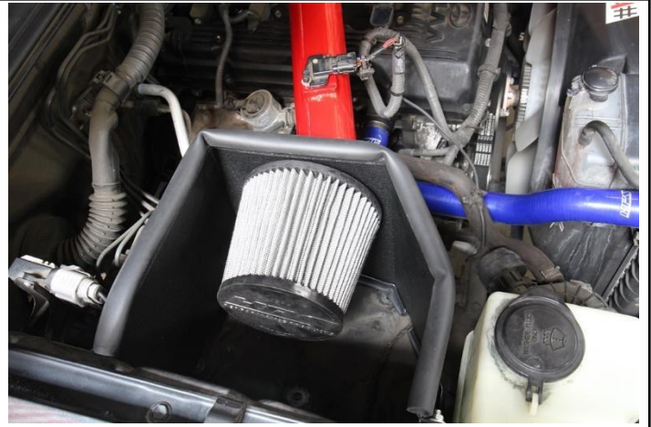
27. Install the provided HPS performance air filter onto the intake pipe.
