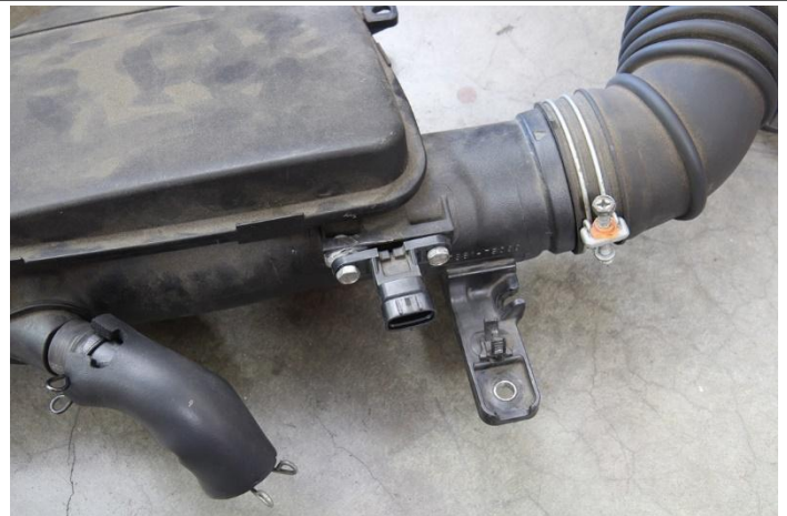
13. Remove the pressure sensor from the stock intake tube.
