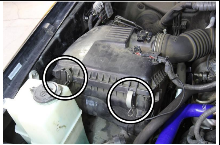
5. Release the two retaining clips securing the upper air box assembly.
