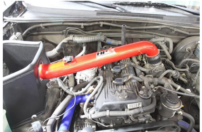
23. Insert the HPS intake pipe into the silicone coupler.
