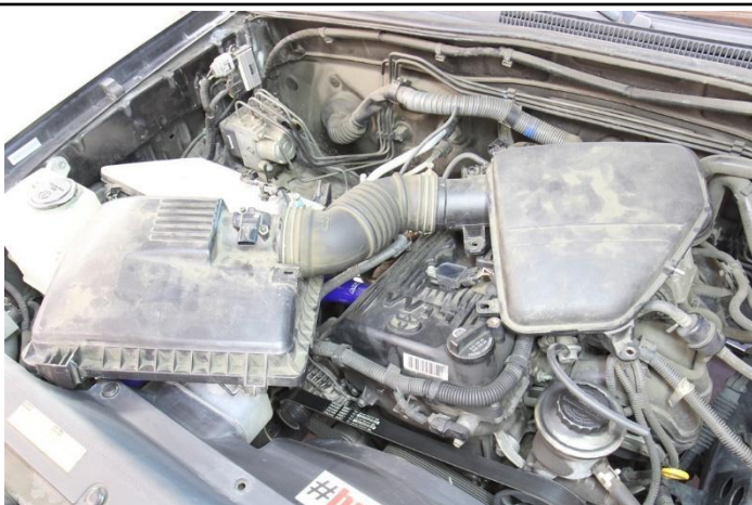
8. Remove the upper air box / intake assembly from the vehicle.
