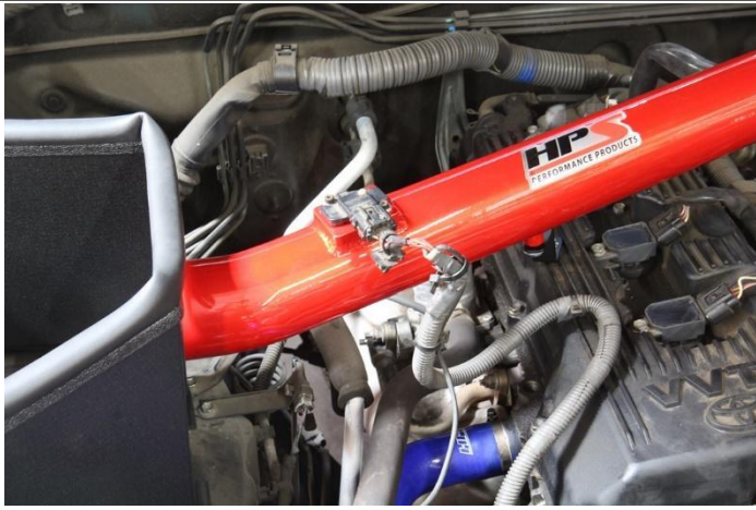
26. Re-connect the MAF sensor harness connector to the MAF sensor.
