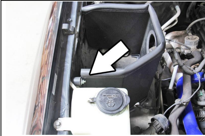
20. Secure the other heatshield mounting bracket onto the vibration mount with a nut and washer.
