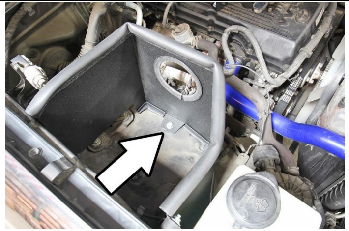
21. Secure the last heatshield mounting bracket onto the stock air box mounting hole by re-using the bolt securing the lower air box removed from step 9.
