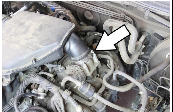
7. Loosen the clamp securing the intake from the throttle body.
