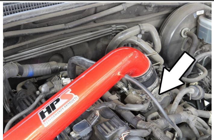
25. Install the provided 4mm vacuum hose onto the intake barb and insert the 16mm vacuum hose onto the other intake barb.
