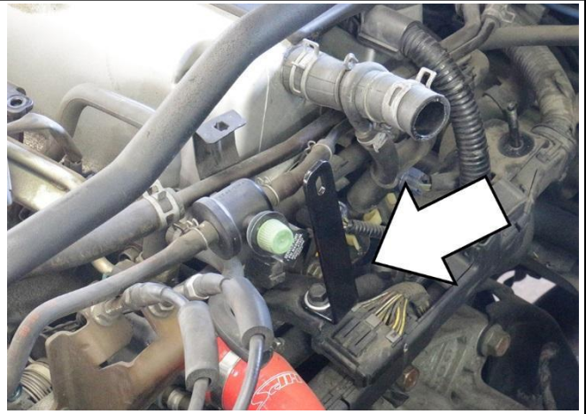
13. Install the intake bracket as shown using a M6 bolt and washer provided in the intake kit.
