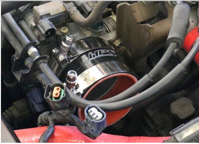
12. Install the silicone coupler onto the throttle body using the T-bolt clamps included.
