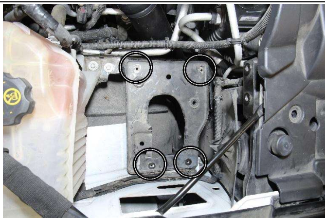
8. Remove the four bolts securing the air box bracket and remove the bracket from the vehicle.
