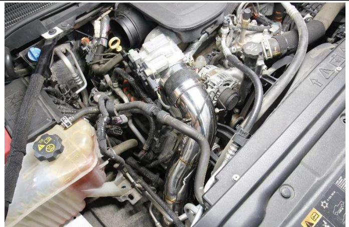
17. Insert the charge pipe into the throttle body coupler. Adjust the charge pipe into position and secure all the t-bolt clamps. Re-connect the air temperature sensor electrical harness.
