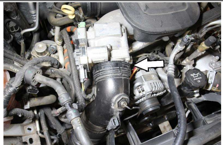
11. Using a flat head screwdriver, rotate the locking mechanism counterclockwise to release the charge pipe from the throttle body.
