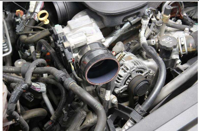
15. Install the remaining reducer coupler onto the throttle body along with the provided t-bolt clamps.
