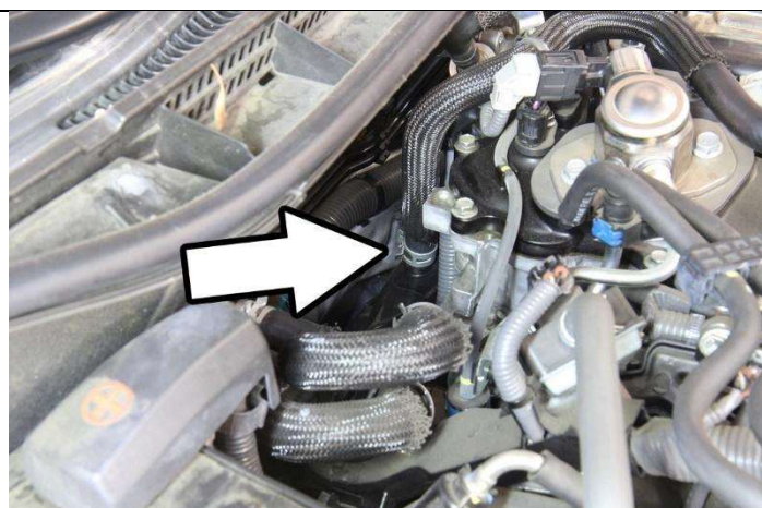
7. Loosen the hose clamp securing the breather hose from the charge pipe and disconnect the hose from the barb.
