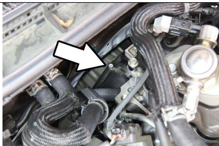
9. Loosen the hose clamp securing the coupler from the charge pipe.
