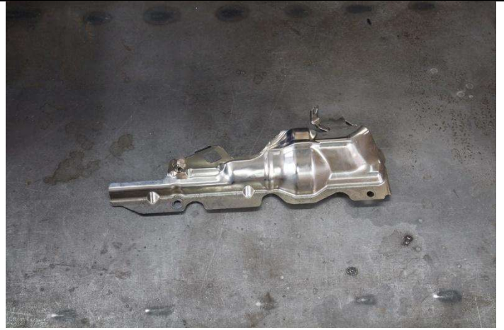
11. Carefully remove the heat shield from the engine.
