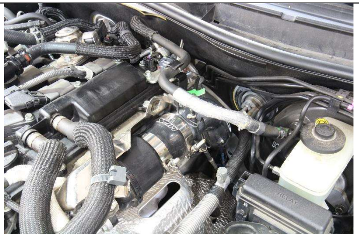
25. Reattach the brake booster hose and the O2 sensor harness connector.
