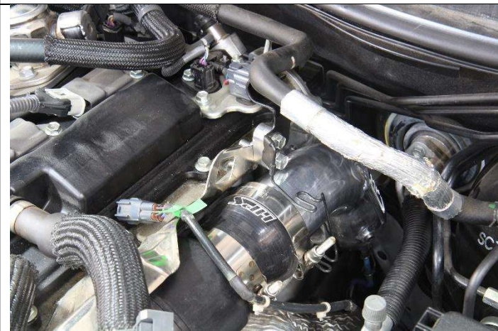
24. Install the assembled brackets onto the heat shield using the original 12mm bolt.
