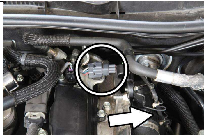
4. Disconnect the o2 sensor electrical harness connector and remove the harness from the bracket.
