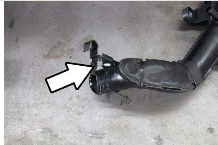
22. Remove the factory upper O2 sensor harness/brake booster hose bracket from the charge pipe.
