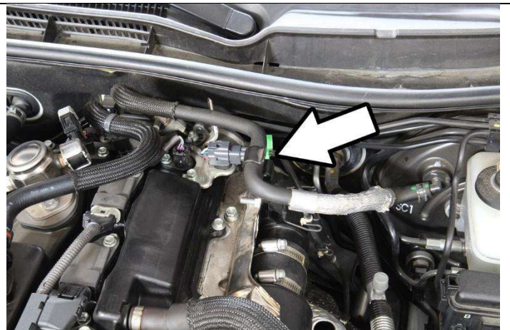
3. Disconnect the brake booster vent hose from the bracket.
