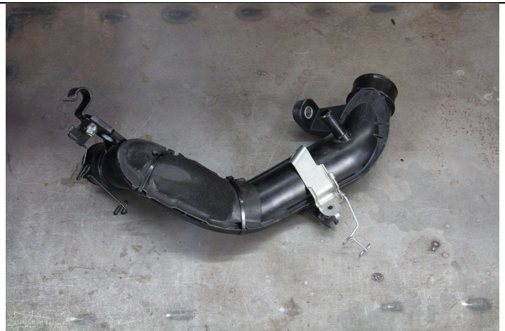
13. Remove stock charge pipe from engine bay.
