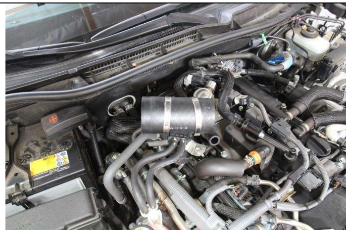
14. Loosen the hose clamp securing the coupler to the heat exchanger and remove the hose from the vehicle.
