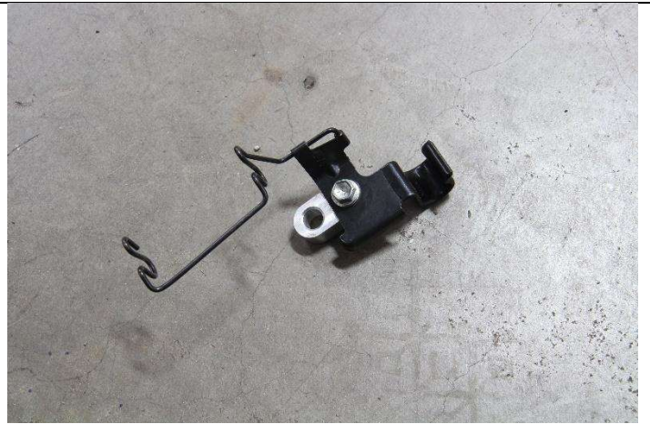
23. Fasten the stock O2 sensor harness bracket/ brake booster hose to the provided bracket reusing the factory 10mm bolt.
