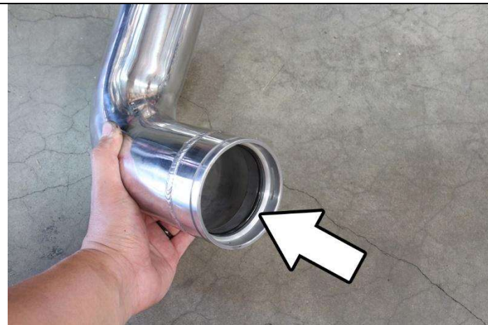
13. Insert the provided O-ring into the HPS charge pipe #2 quick connect.
