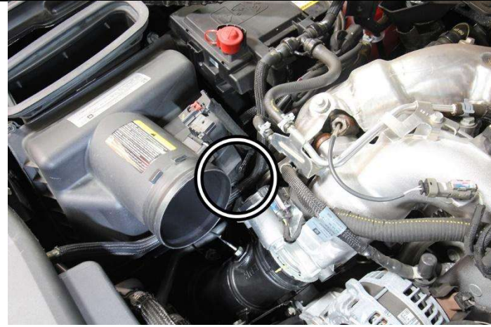
4. Disconnect the coolant hose clip and the MAF sensor harness clip from the air box assembly.
