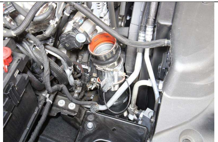
18. Insert the HPS charge pipe #1 into the charge pipe #2 until the coupler hits the sensor bracket.
