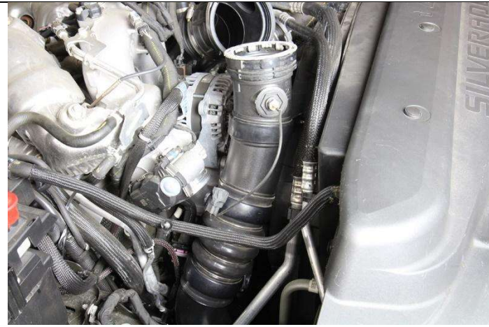
9. Remove the cold side intercooler tube assembly from the vehicle.
