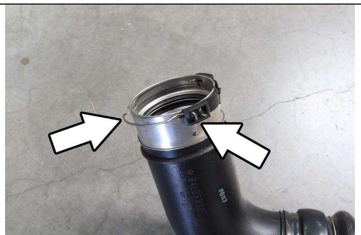
8. Lift up both sides of the retaining clip using a flat head screwdriver to loosen and remove the intercooler tube from the intercooler side.
