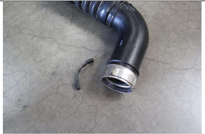
16. Once the plastic clip is removed you can now remove the metal retaining clip from the stock charge pipe.
