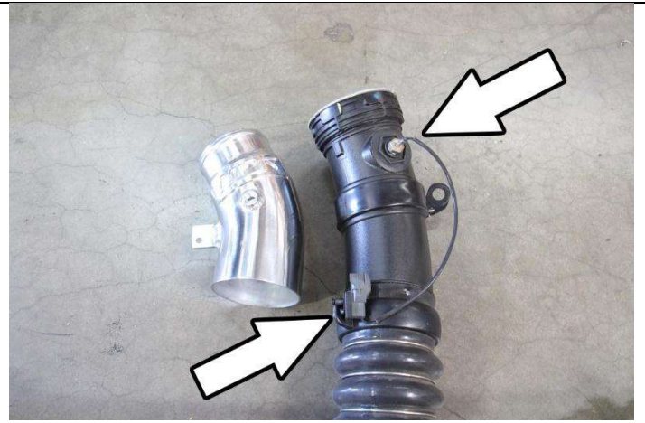
10. Using a 14mm open wrench, loosen and remove the temperature sensor and electrical harness from the stock charge pipe.
