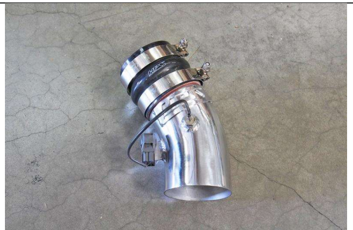
12. Insert the hump coupler along with the provided t-bolt clamps onto the HPS charge pipe #1.
