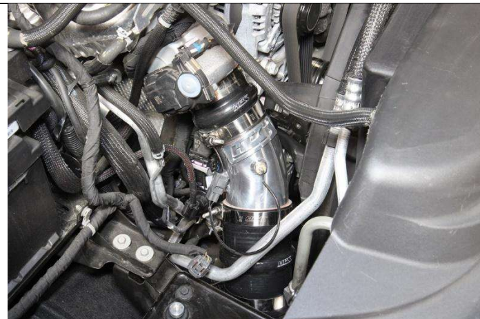
19. Rotate the charge pipe and insert the coupler onto the throttle body. Secure all the hose clamps once the charge pipes are properly positioned..
