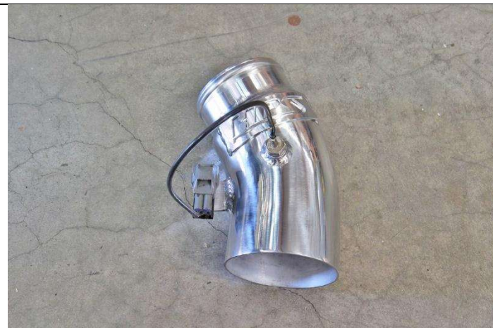
11. Install the temperature sensor onto the HPS charge pipe #1.
