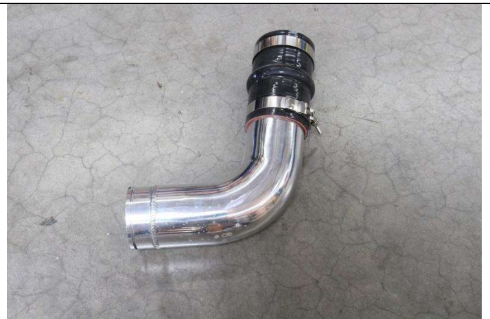
14. Install the 6-inch hump coupler along with the provided T-bolt clamps onto the charge pipe #2.
